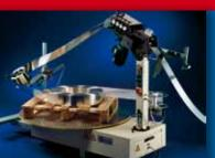
Single, double or triple pallet decoiler with strip-straightener. Load capacity < 3000 kg.
