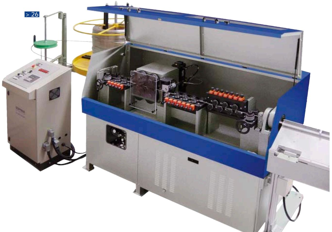
Modern production companies automate wire feeding with decoilers, straightening-feeding systems and cut-to-length lines.
