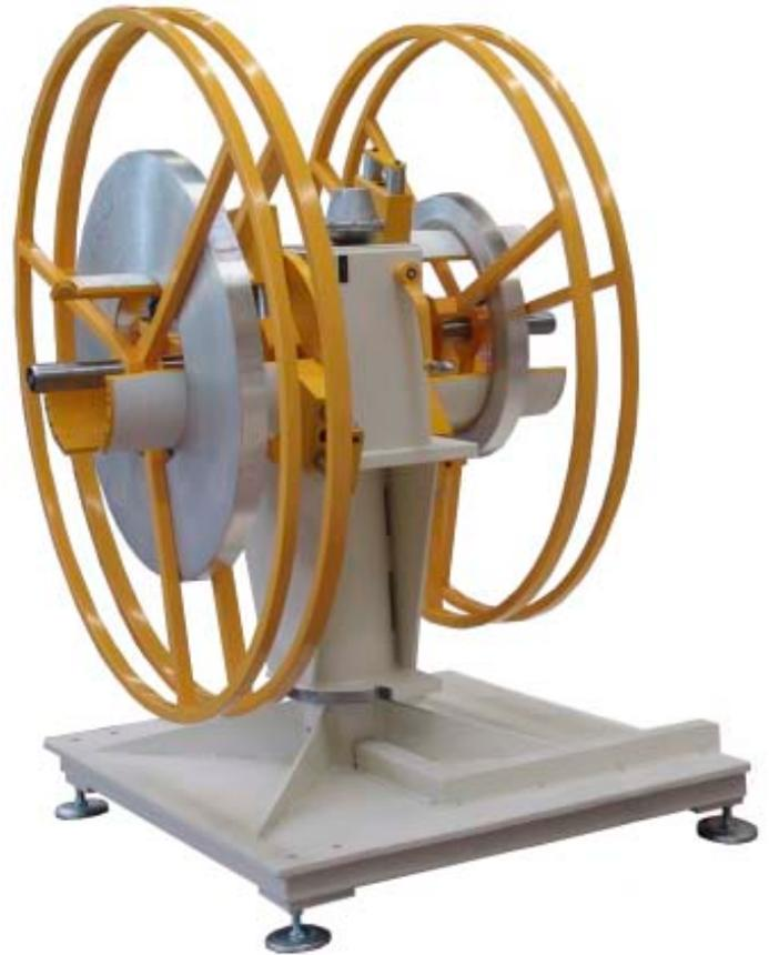
Our decoilers/rewinders are equipped with various mandrels to suit the respective requirements. Precision mandrels with centrally adjustable coil clamping are being used increasingly. This version is kind on the edges of thin and narrow strip and guides it accurately. Decoilers/rewinders for horizontal coil handling as well as for processing of carrier bobbins, also with traversed strip, round off our range.
