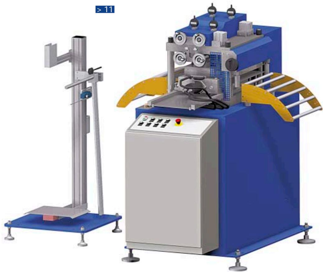
More and more often, the punching industry uses a motorised strip straightener in front of the press. Straightening conserves tools thereby producing more accurate components. As the strip is fed over a loop into the feeder without any pulling force, higher production rates can be achieved.
